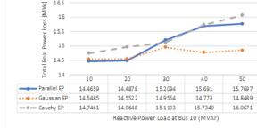
Total Power Loss vs Reactive Load Variation at Bus 10
